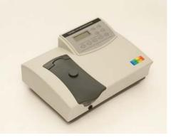
This is the latest addition to our M100 Series of Visible Spectrophotometers. The replacement of the manual wavelength/filter control knob of the popular M107, by processor controlled stepper motors allows a step change in capabilities. The M108 has a 4 line x 20 character display and a 9-button keypad to allow easy use and full access to this intelligent spectrophotometer.
